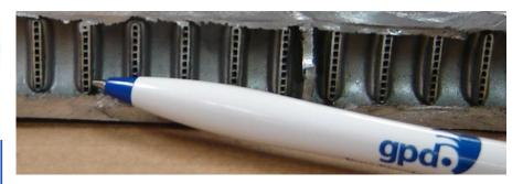
When a compressor fails it introduces contaminates into the system, one of the easiest ways to spot this is to remove the orifice tube that usually reveals metal deposits or sludge from a faulty compressor. The metal and sludge gets deposited throughout the system and will collect at places in the system with restrictions, like the orifice tube and on later model vehicles, the parallel flow condensers.
