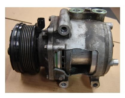
When confronted with a compressor failure on a vehicle fitted with a parallel flow condenser, we recommend that the technician replace the accumulator, orifice tube or expansion device and condenser. We also recommend that all other components are flushed to ensure they are free of contaminates that could harm the new compressor.
