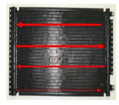
In a parallel flow condenser, the refrigerant changes direction by 180° at the end on the side rails by placing a plug inside the rail at intervals, forcing the refrigerant change directions. The more plugs, the more times the refrigerant changes direction. In most condensers, the refrigerant makes three to four "passes" through the condenser.
